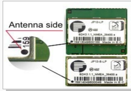
Figure 6: JP13-LP/LPx & JP13-S-LP/LPx orientation point for antenna site.
