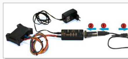
Figure 1: Use the Control-box for connection of a FOX3-2G/3G/4G series device to a PC
