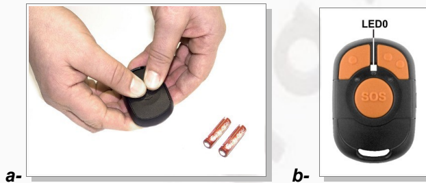
Figure 7: Inserting included batteries in Keyfob.
