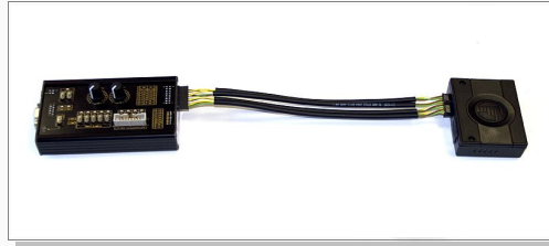
Figure 8: I/O-BOX connect to I/O-BOX-EVALBOARD via 16-pin MOLEX cable.
