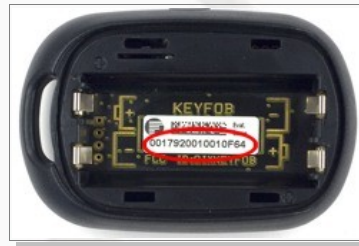
Figure 4: The location of MAC address on Keyfob.
